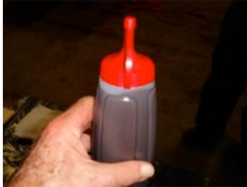
Pour the **well stirred oil** into a handy squeeze bottle. This will allow you to control the amount of oil you want on the floor. We stock these and will include one with each order **Do not flood the floor with the oil. Instead use an absolute minimum of oil.** Just enough to get thorough coverage of the surface.
